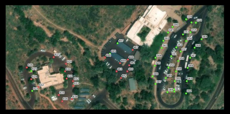
Example of IDA compliant (green dot) and non-IDA compliant exterior lighting fixture analysis at a Park Service location. Within the GIS-based collection system, fixture characterization data (including photos) collected in the field are automatically stored in the cloud for later processing. Each point is a live link to the data that partners can later access via GIS software, ArcGIS Online, an interactive Story Map or Dashboard, or through other technologies.
