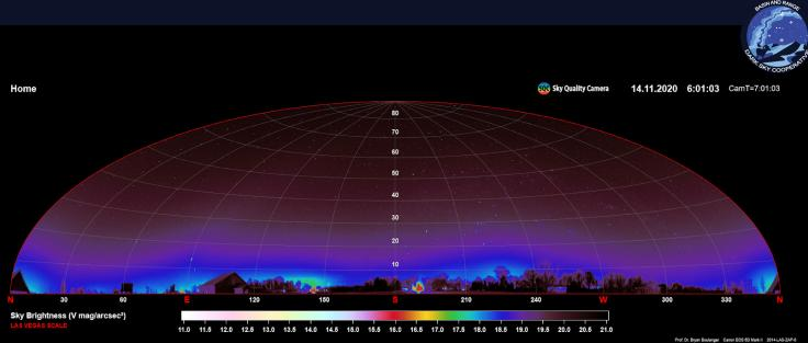
Example of photometric analysis for sky brightness near Bryan's home in Ohio Northern University. The image shows sky brightness measured in visual magnitude per arc second area. This unit is the same measurement unit reported by Sky Quality Meters. However, here the camera system maps sky brightness from the horizon to the zenith over a 360° view surrounding the camera. Light domes on the horizon are clearly visible.
